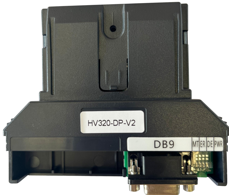
Figure 1-1 Appearance of the HV320-DP-V2 card
